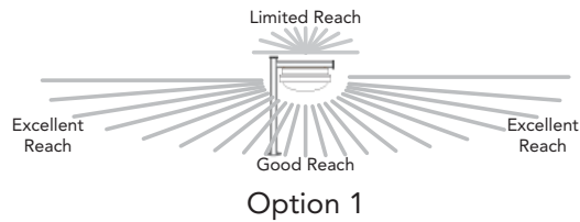
Figure 2: Typical AP internal omni coverage, side view
